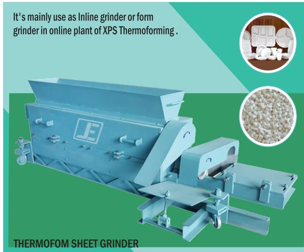
It's mainly use as Inline grinder or form grinder in online plant of XPS Thermoforming .
