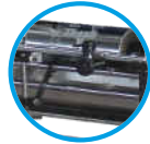
360° Universal Movement Oscillating Doctor Blade
