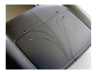
Causes: Flow line defects are caused by the varying speed at which the molten plastic flows as it changes direction through the contours and bends inside the mold tool. They also occur when the plastic flows through sections with varying wall thickness, or when the injection speed is too low causing the plastic to solidify at different speeds.
