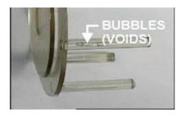
Causes: Vacuum voids are often caused by uneven solidification between the surface and the inner sections of the prototype. This can be aggravated when the holding pressure is insufficient to condense the molten plastic in the mold (and thereby force out air that would otherwise get trapped).
