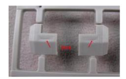
Causes: Sink marks are often caused when the cooling time or the cooling mechanism is insufficient for the plastic to fully cool and cure while in the mold. They can also be caused by inadequate pressure in the cavity, or by an excessive temperature at the gate. All else being equal, thick sections of the injection molded part take longer to cool than thin ones and so are more likely to be where sink marks are located.
