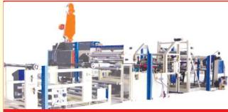
**Extrusion Lamination Plant For Paper**
