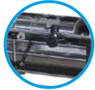
360° Universal Movement Oscillating Doctor Blade
