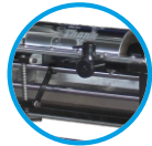
360° Universal Movement Oscillating Doctor Blade
