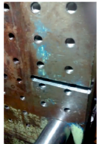
3. Cut slot by the end-mill cutter
