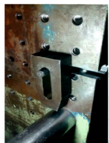
9. 'T-bolt' with clamp in the newly made 'T-slot'
