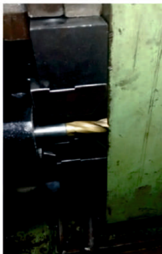
2. Starting the cutting of material of patten with end-mill cutter
