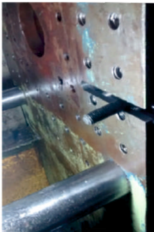
7. 'T-bolt' slide to the center of 'T-slot'
