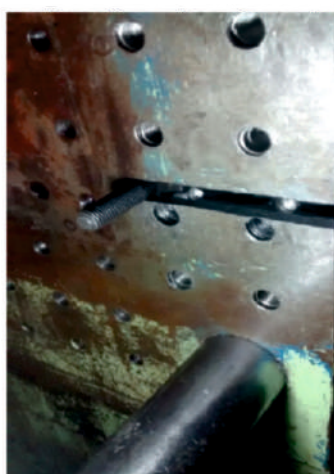
8. 'T-bolt' slide to the end of the 'T-slot'
